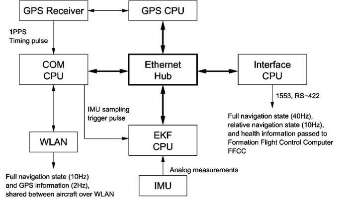
Fig. 1. FFIS hardware block diagram.
