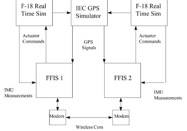
Fig. 2. FFIS HIL Sim block diagram.
