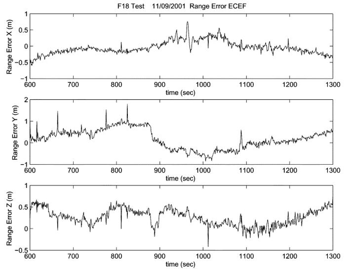
Fig. 4. Relative range estimate from the EKF—F-18 test.
